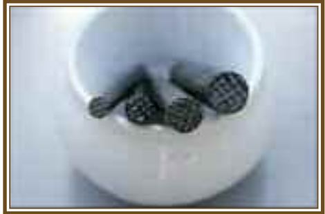
The serrated ends of the punches
