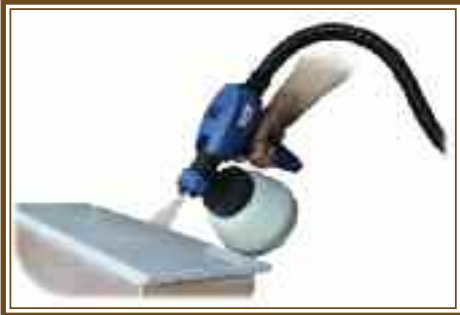
Applying varnish with a spray gun
