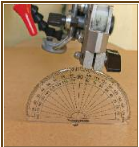
Figure 5. Setting the Sawing Angle
