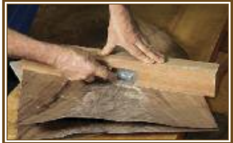
Cutting the book match pair with a veneer saw and straight edge
