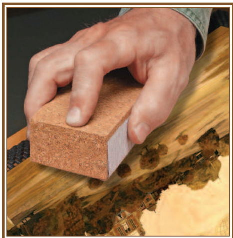
Sanding with fine grade abrasive papers wrapped around a cork block using smooth, light strokes.
