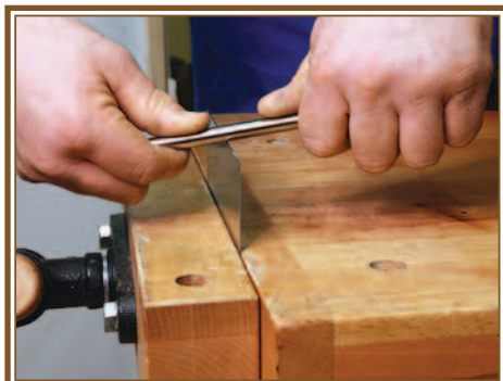
Using a burnisher to form the cutting burr (or cutting lip)
