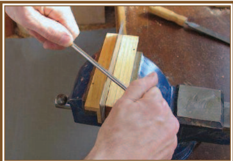
Forming the cutting burr
