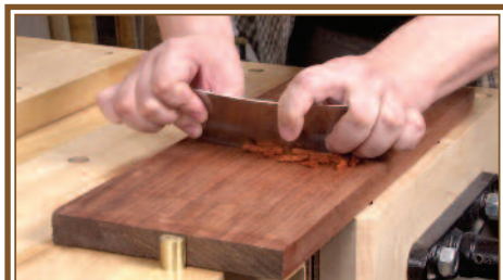
Showing a cabinet scraper in use
