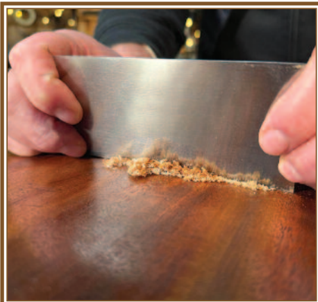
The cabinet scraper used the correct way
