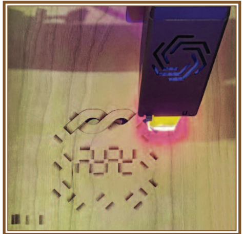
The laser cutter burning the Celtic Knot design after first burning the sand scorch elements of the design
